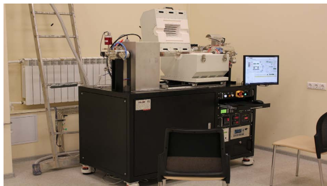
Figure 3 – General view of the chemical vapor deposition plant (the furnace is open and in the non-working position)
